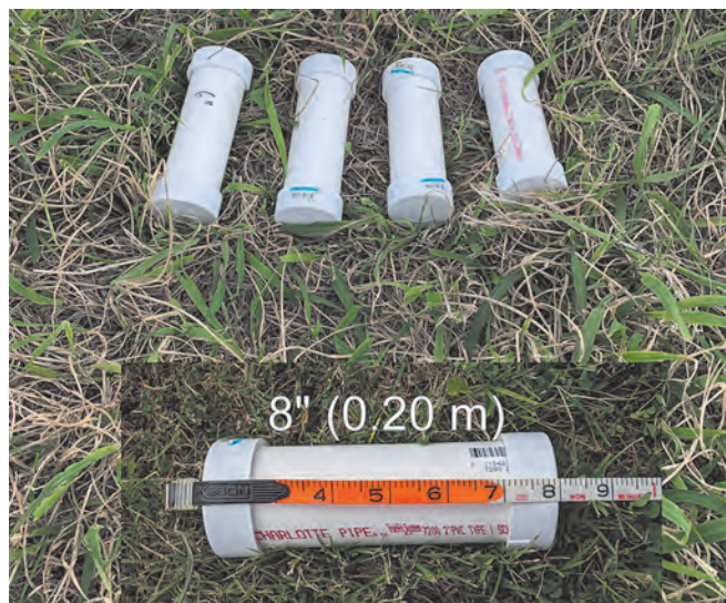
Figure 6. Four reference markers filled with steel nails were installed in the four corners of the GTS.
