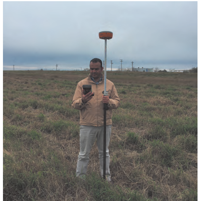
Figure 2. Topographic survey using GPS before the GTS construction.
