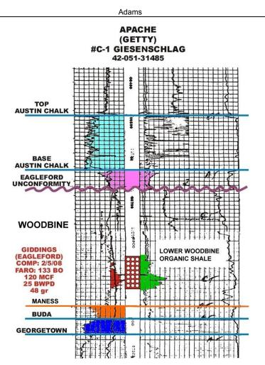
Figure 9. Type log of LWOS in Brazos and Burleson county area. In the study area, we are mapping only the interval with both the hot gamma ray and the higher resistivity.
