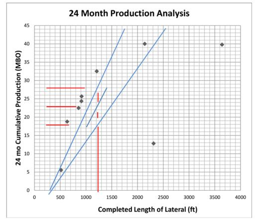
Figure 12. Graph of 24 mont cumulative production versus completed length of lateral for 9 short Apache horizontal wells completed in the LWOS. Average production is 23,000 BO per 1000 ft of lateral for the first 24 months.
