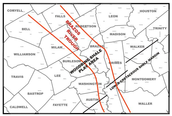
(TROUGH INTERPRETED TO DEPTH TO MAGNETIC BASEMENT)
