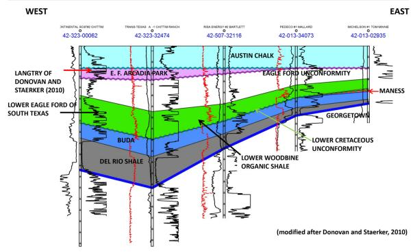
Figure 7. Cross-section 4. West to east cross-section extending cross-section 3 into the Maverick Basin. Note the thickening of the LWOS into the Maverick Basin and the appearance of true Eagle Ford (Langtry of Donovan and Staerker, 2010). The LWOS is clearly equivalent to the Lower Eagleford/ Eagle Ford of South Texas terminology.
