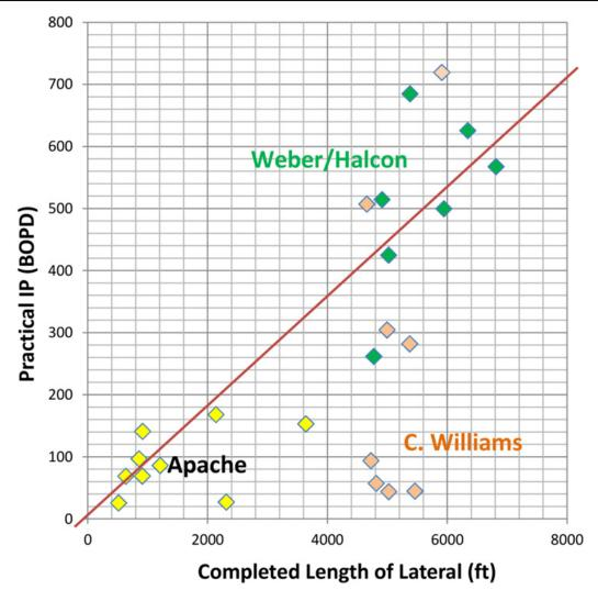
Figure 19. Practical IP versus completed length of lateral of Figure 18 plus 8 wells by C. Williams and the first 7 wells by Weber/Halcon. Note that most wells except those by C. Williams fit this graph.
