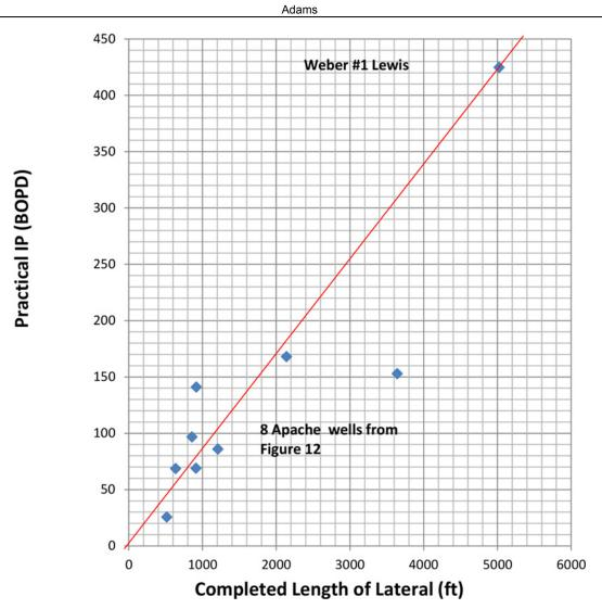
Figure 18. Practical IP versus completed length of lateral for the 8 Apache wells in Figure 17 plus the 2012 completion in the Weber #1 Lewis well in northern Brazos County. The #1 Lewis well has a 5021 ft completed lateral and demonstrated that this analysis can be upscaled.
