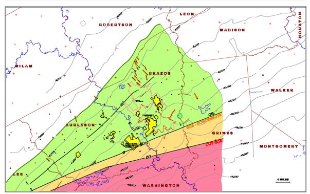
Figure 13. Map of produced oil gravity from the LWOS across the study area. 50 degree gravity is used here as the arbitrary boundary between the oil and gas-condensate windows.
