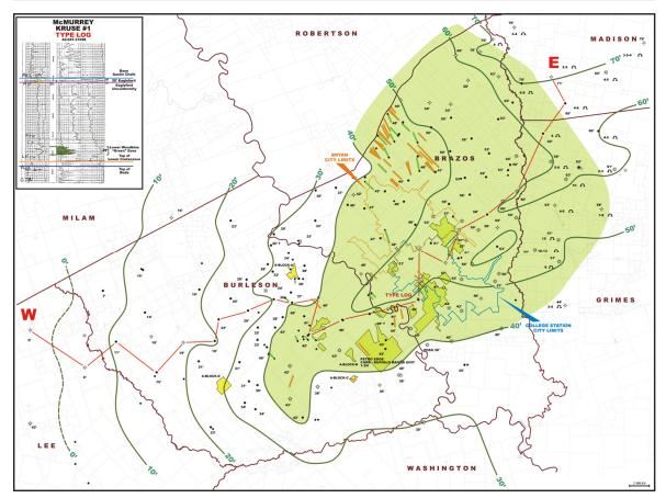
Figure 10. Interval isolith of the LWOS in the study area. Note that the interval goes to zero to the west. To the east, the edge of the green shaded area represents where the interval is losing both resistivity and gamma ray signature. To the west, the interval is replaced vertically with a resistive shale without the hot gamma ray signature.
