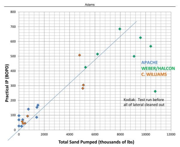
Figure 20. Practical IP versus total sand pumped for the same wells shown in Figure 19. Note the better fit when total sand pumped is used instead of length of lateral.
