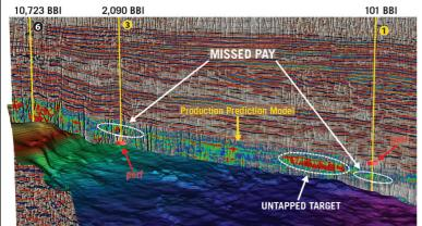
An arbitrary line through 3 vertical wells in the West Texas Permian Basin shows the lateral variations of the Production Prediction Model and reveals refrac potential for Wells 1 and 3 where the red disks indicate the actual completion intervals and the white circles highlight the missed pay. Note the untapped target near Well 1.
